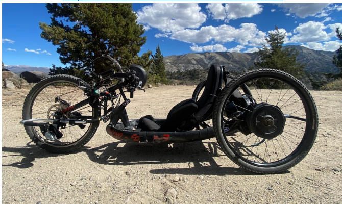
Top End Force 3 with dual rear motors
